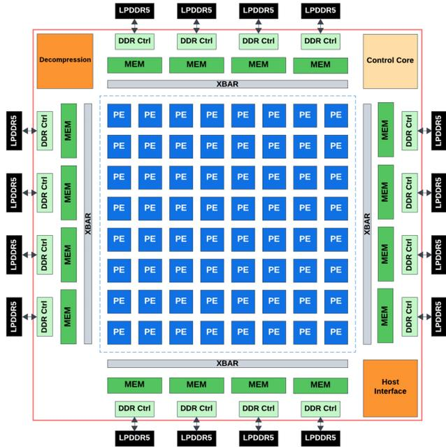
Figure 1: MTIA 2i's overall architecture.
